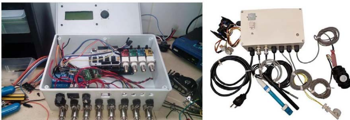
Figure 10. Organization and location of the hydroponic farm sensors.
